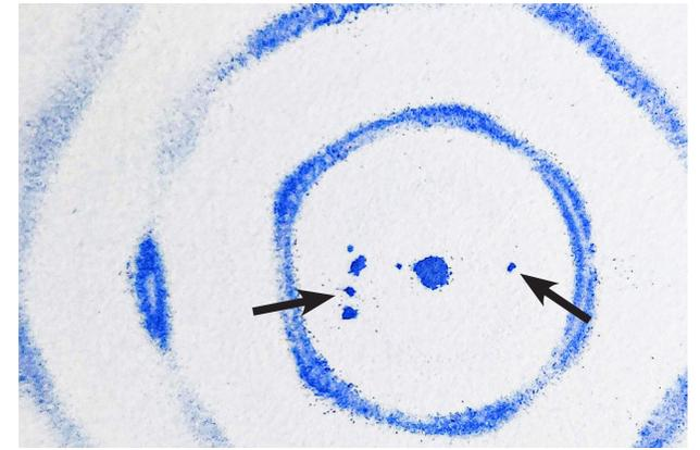
Fig. 9: Spots form at nodes where droplets coalesce.
